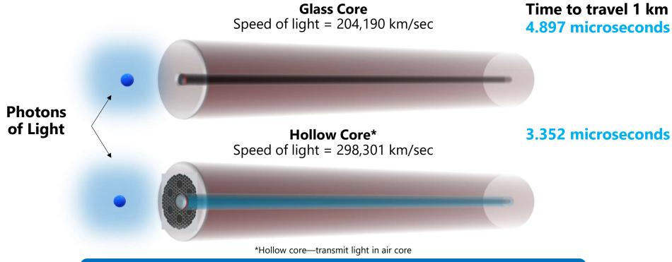
The Challenge: to realize the latency improvement in field deployed networks because the fiber (i.e., hollow core) is intrinsically sensitive to external stress.
