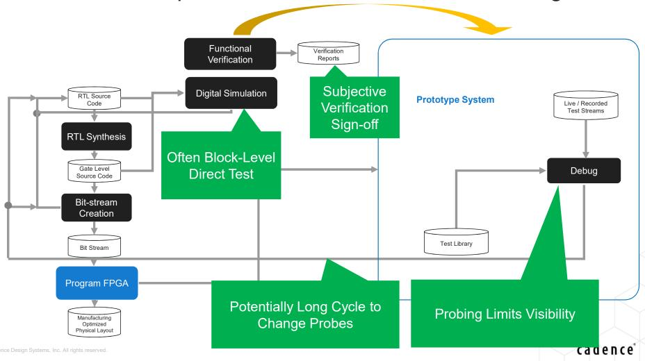
Detailed FPGA Development Flow With Quantitative Analysis
