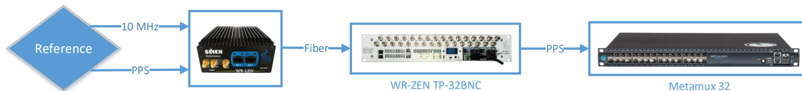
Metamako Synchronization offset using PPS
