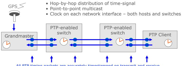
All PTP timing packets are accurately timestamped on transmit and receive
